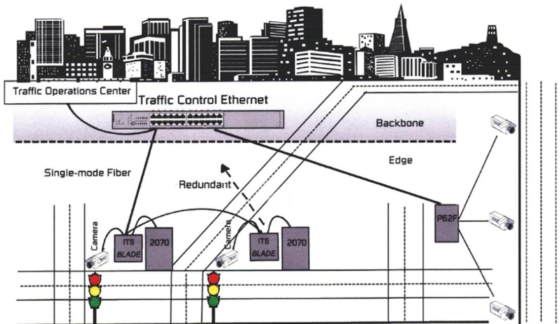
The active hardware in a complete Ethernet IP-switched network solution is roughly one-half the cost of a combination T1 and SONET or ATM solution, and provides about 10X greater bandwidth for the video data as well.
