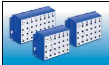
The new Hirschmann OCTOPUS 30/34 switch features four Gigabit Ethernet (GE) ports (available in copper or fiber), L3 routing functionalities and Power over Ethernet (PoE) support for maximum network availability. It also includes the latest bypass relay feature as specified in IEC EN 61375 for reliable networking.
