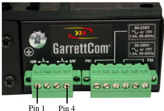
Fig 3.5a Alarm Contacts: (1,2) hardware controlled (3,4) software controlled
