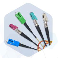
Belden's Fiber Express (FX) Fusion Splice-On connectors combine the benefits of fusion splicing with the simplicity of a field-installable connector to expand your options for field termination and improve installation performance and reliability over mechanical splice connectors. No crimping, polishing or adhesives are required for termination, minimizing installation errors.
